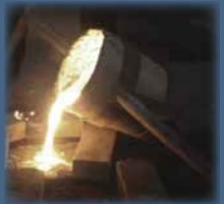
Pouring molten brass into a mold.
