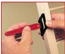
Centering/Parallel Guide Fits Up to 3/4" Thick Trailing Edges
